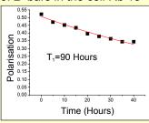
polarisation decay over time we calculated a <sup>3</sup>He relaxation time (T1) of 90 hours in the ILL "Magic box." All values were produced using the "Poltax" fitting software.
